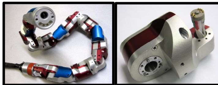
Fig. 1: The Unified Snake robot (left) and one of the individual 1-DOF modules from the snake robot (right).
