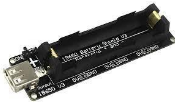
Fig. 23: Image of 18650 Battery shield showcasing its multiple output options.
