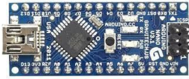
Fig. 26: Top view of Arduino Nano showcasing its pin layout.
